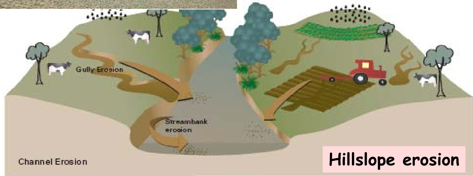
Illustration of channel and hillslope erosion processes. Channel erosion includes gully and streambank erosion and hillslope erosion includes sheetwash and rill (shallow [ <20 cm] channel) erosion.
