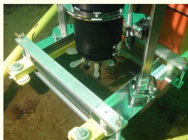
Vertical profiles of dissolved oxygen micro-electrodes (resolution of 100-200  $\mu\text{m}$ ) are obtained together with resistivity and pH measurements. The measuring electrodes are moved vertically by a pre-programmed motorised system.
