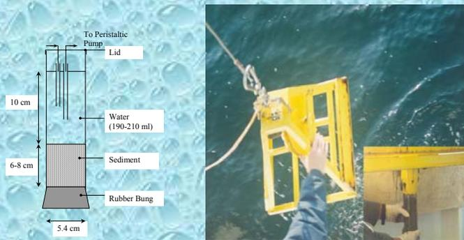
Experimental incubation design. Triplicate sediment cores and a control of water only were used for nutrient flux assessment. All cores were maintained in a water bath at *in situ* temperature in darkness.
