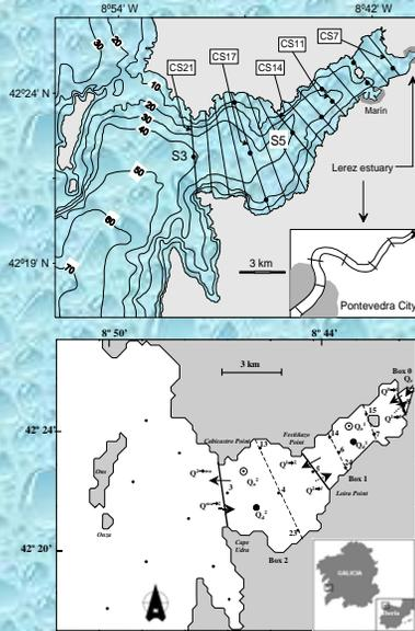
An analysis of the intra-annual variability of hydrographic residence times,  $\tau$ , quantified with an iterative approach to the fraction of freshwater method using 23 quasi-steady state water-salt budgets. Mean  $\tau$  was  $6 \pm 2$  d in the central ria and  $2 \pm 1$  d in the internal ria. The tidal contribution, equal to 10-25 % of total water renewal, was quantified for the first time for a Galician ria with the hydrodynamic model ECoS. *Dale et al. (2004)*
