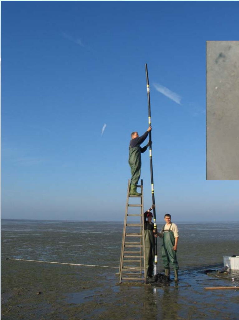
installation of permanent in-situ pore water sampler
